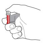
15. Snap cap fully onto tube.
